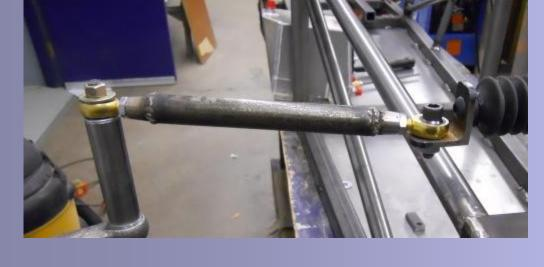
We were able to get help on the ball-joint mounts. After this we were able to move forward on front wheel assembly. Instead of attaching the ball-joints to control arms, we connected them directly to the frame. We also finished the steering components. Instead of trying to reuse go-cart tie rods, we made our own, using 3/4" tube and threaded inserts.
